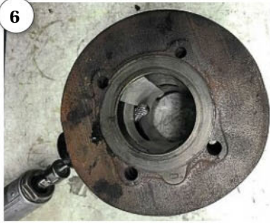
6: Use masking tape as guidelines and ream port 1mm at top and sides. 7: Port done, ready to be chamfered.
