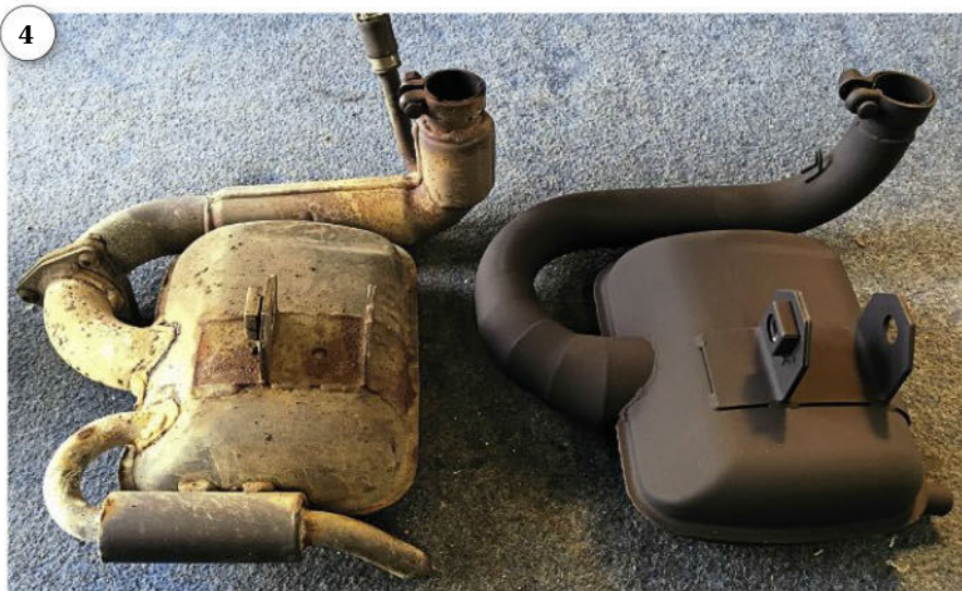
4: Side-by-side: the emissions-friendly and functional exhaust on the left, SIP performance item on the right. 5: LML Star available for a quick comparison.
