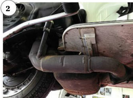
1: Basic 125 lump, prime for fettling. 2: On this side the breather pipe needs unscrewing and the 13mm stub-bolt slackening. 3: On this side the 17mm bolt runs through the frame. Deflate the rear tyre to assist with removal.
