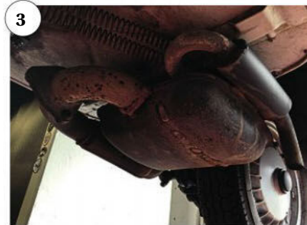
1: Basic 125 lump, prime for fettling. 2: On this side the breather pipe needs unscrewing and the 13mm stub-bolt slackening. 3: On this side the 17mm bolt runs through the frame. Deflate the rear tyre to assist with removal.
