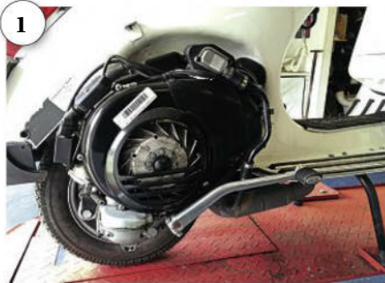
1: Basic 125 lump, prime for fettling. 2: On this side the breather pipe needs unscrewing and the 13mm stub-bolt slackening. 3: On this side the 17mm bolt runs through the frame. Deflate the rear tyre to assist with removal.
