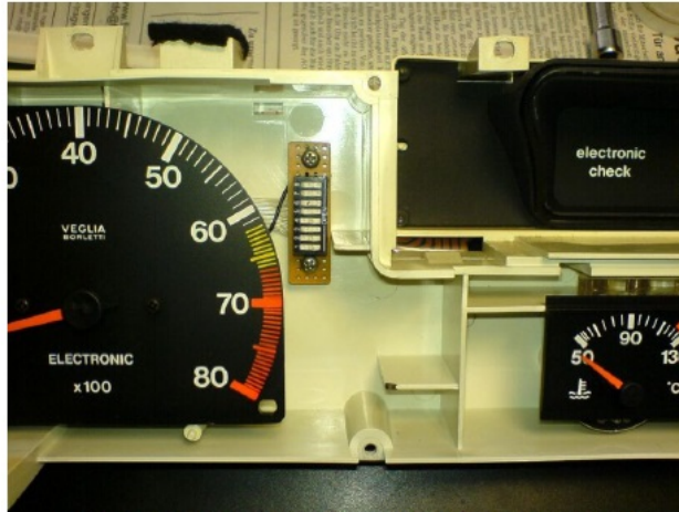
Fig 3. Example of DIP-switch installation in Fiat Tipo 2.0 16v instrument cluster
